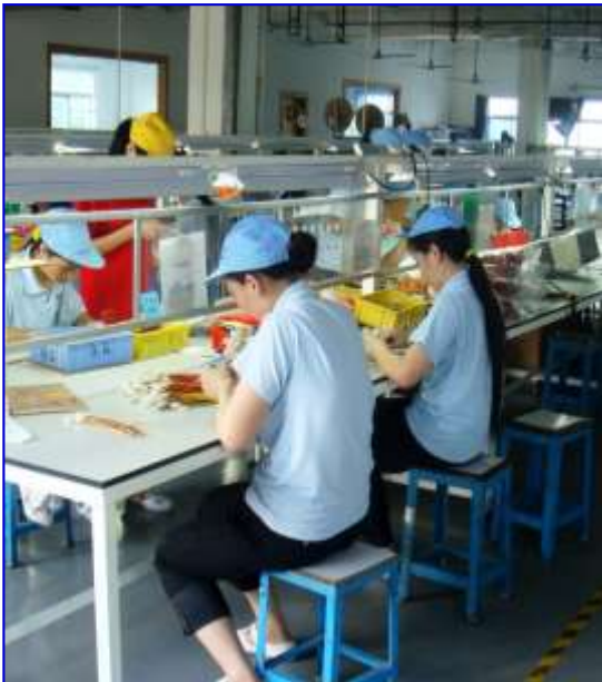
Operators conducting Visual Inspection
