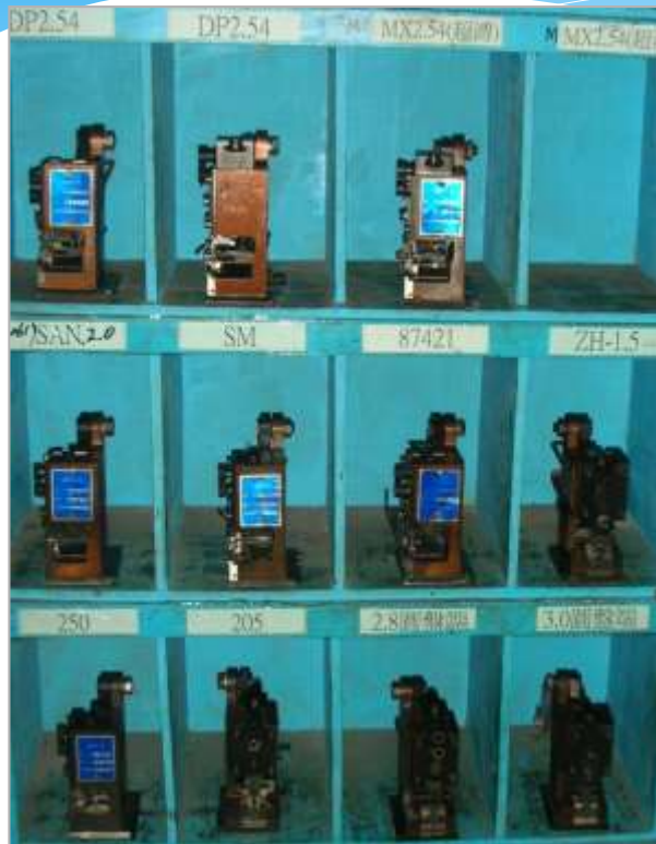
Applicators Rack ( Storage Area )
